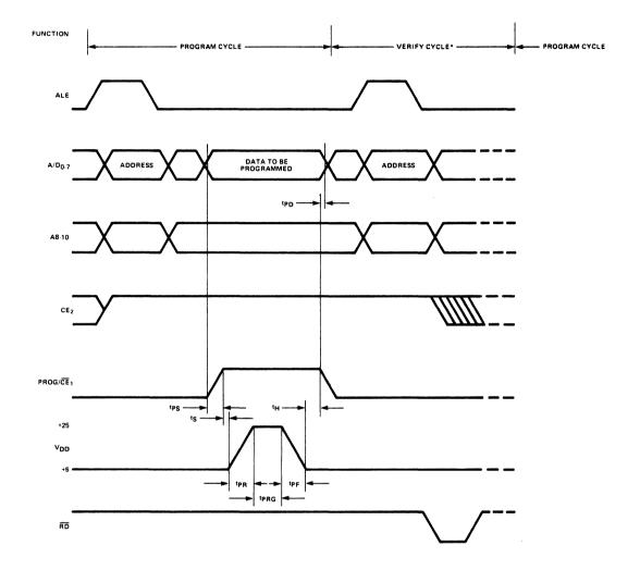
\*VERIFY CYCLE IS A REGULAR MEMORY READ CYCLE (WITH VDD = +5V FOR 8755A)
